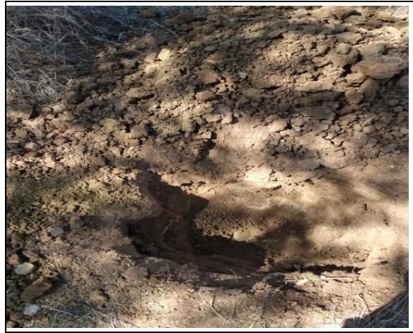
FURO 28 –. ST-28 - Argila compacta (0,80m)
