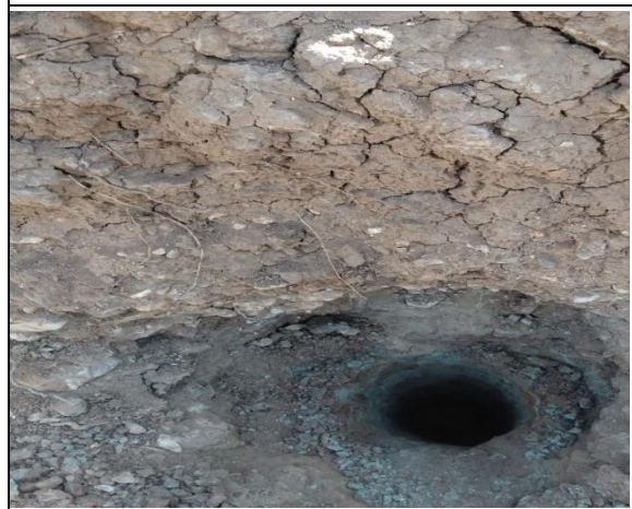
FURO 26 –. ST-26 - Silte argiloso (1,80m)
